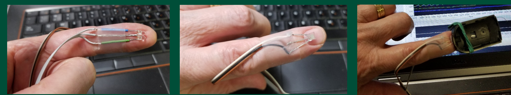
Figure 2. My finger with attached blue and green LEDs (left), photodetector (center), and plastic cover secured by a rubber band.
