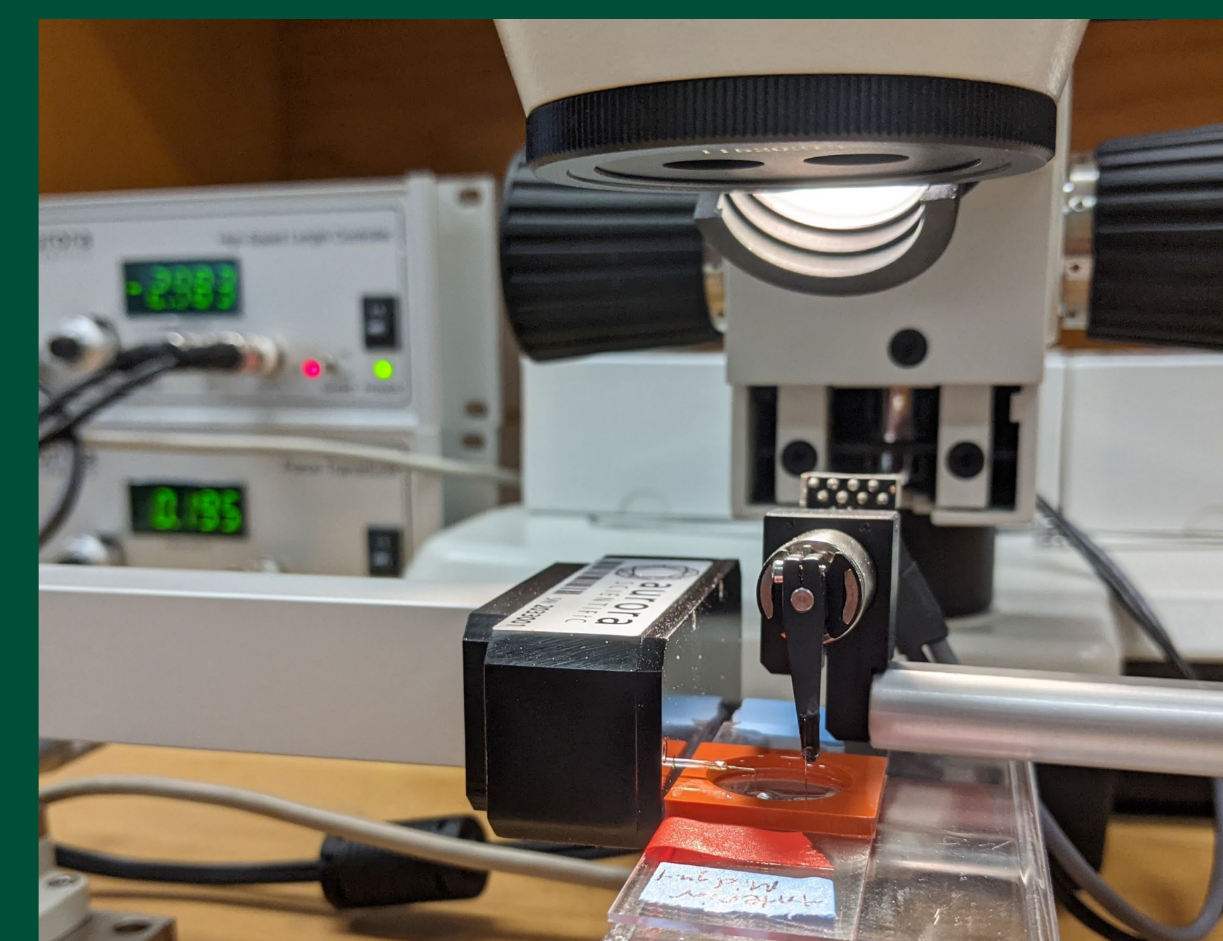
Figure 2: Our lab's soft matter linear extension instrument, mounted on a light microscope.
